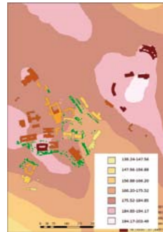
Solar Radiation Flux (mW per m 2 ) calculated for Keele Campus showing buildings (pink and white) with high potential for Solar PV. From the MSc thesis of Ms U. Weerakody (2011)
